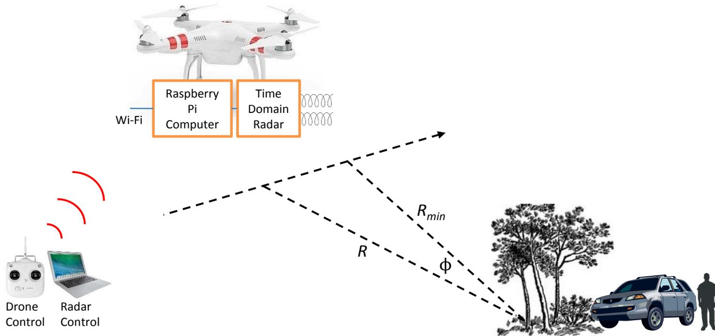
SAR system consists of P410 radar, Raspberry Pi + Wi-Fi Dongle, helix antennas mounted on aluminum ground planes. Entire system (including cables and batteries) weighs less than **300 g**.
