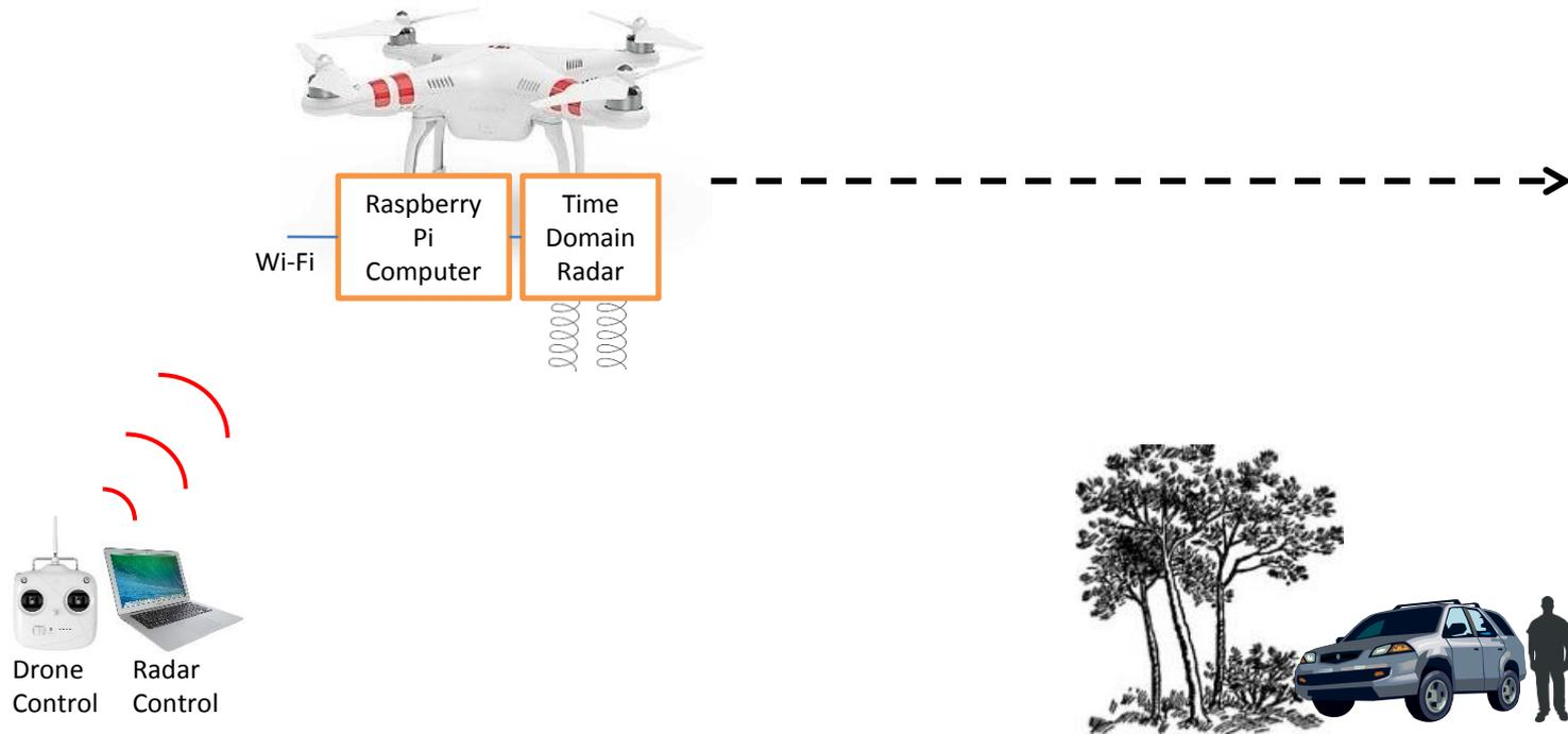
Point antennas at the ground in order to change imaging plane.
